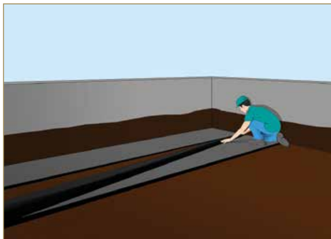
Figure 7.14: Fold and adhere the second half of the membrane
