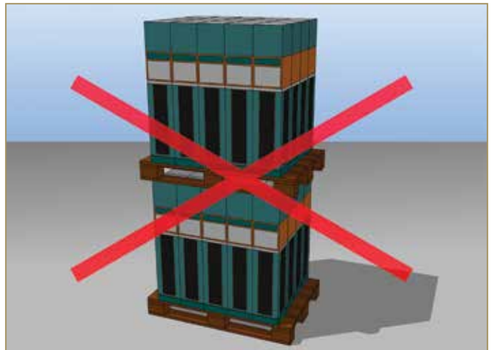
Figure 6.2: Avoid stacking two or more pallets
