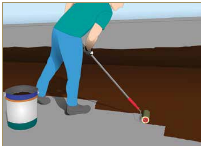
Figure 7.1: Application of the primer
