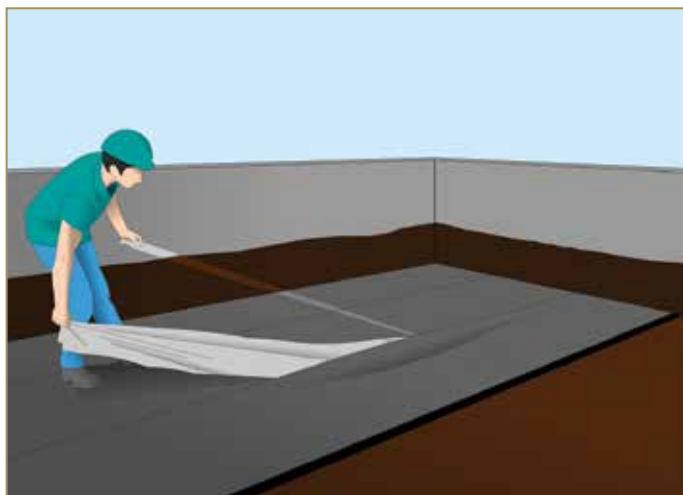
Figure 7.15: As an alternative to Figure 7.11 - 7.12 - 7.13 - 7.14 it is possible to remove both halves of the protective film at the same time
