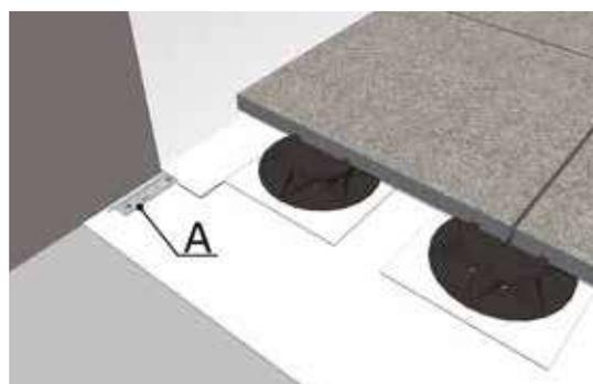
A - Linear mechanical fastening with pre-punched MAPEPLAN METALBAR + MAPEPLAN T CORD + fastening elements (min. 4 pcs/m).
