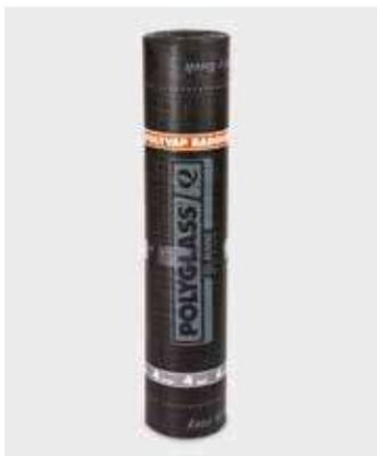
POLYVAP RADONSHIELD P-AL is a prefabricated waterproofing elastomeric-plastomeric membrane, with a distilled bitumen-based compound modified with polypropylene, reinforced with a 6/100 thickness aluminum strip bonded to reinforced glass fiber.
