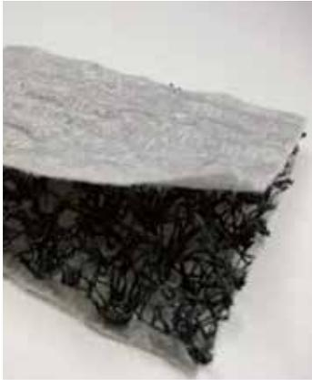
POLYSTUOIA 20 and POLYSTUOIA 20L are protective and drainage geocomposites comprising two UV-stabilized, needle-punched polypropylene staple-fiber filter geotextiles with a 3-dimensional drainage structure sandwiched between them made up of polypropylene monofilaments.
