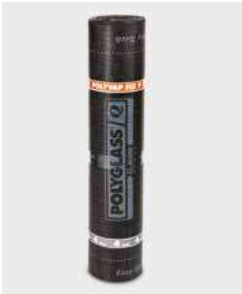
POLYVAP FIX P e POLYVAP FIX P-AL are a prefabricated waterproofing elastomeric membrane. POLYVAP FIX P is a vapor underlay featuring a spunbond polyester nonwoven carrier stabilized and reinforced with glass strands parallel to the machine direction. POLYVAP FIX P-AL is a vapor barrier featuring a glass fiber stabilized polyester fabric carrier laminated with aluminum foil, set within the membrane.
