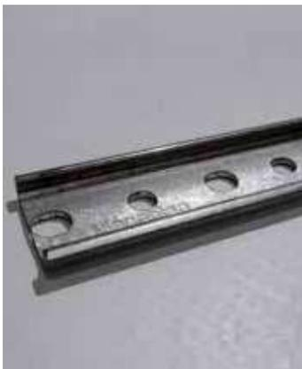
MAPEPLAN METALBAR is a metal fixing profile in galvanized carbon steel, pre-punched, with oval perforations, to be used around the perimeter of the waterproofing membrane to anchor the sheet.
