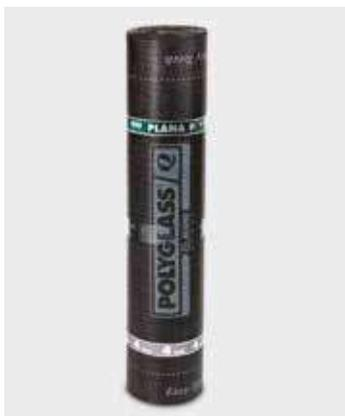
PLANA P is a prefabricated waterproofing elastomeric-plastomeric membrane, with a distilled bitumen-based compound modified with polypropylene and staple non-woven polyester fabric reinforcement.
