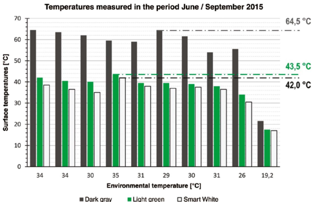
**The MAPEPLAN® T Smart White waterproofing membrane makes a significant contribution to improving building energy efficiency.**
