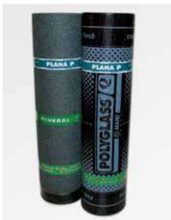
PLANA P is a prefabricated waterproofing elastomeric-plastomeric membrane, with a distilled bitumen-based compound modified with polypropylene and staple non-woven polyester fabric reinforcement.
