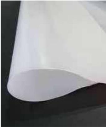
MAPEPLAN VB PE - MAPEPLAN VB PE SD 220 is a vapour control layer in low density LDPE polyethylene. It is used to as vapour control layers and as a functional element in producing build-up systems for warm roofs. Designed to be applied on the “warm side” of the thermal insulation.
