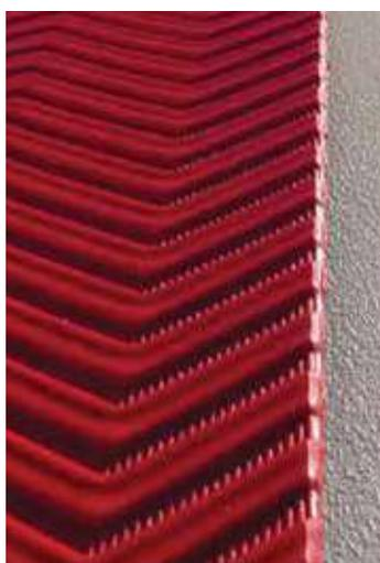
MAPEPLAN T WALKWAY is a FPO/TPO protection rooftop membrane with a composite glass fleece/glass fibre combi reinforcement, produced with a structured non-slip surface making the roof suitable for foot traffic and allowing access for maintenance purposes. Designed to be applied on top of MAPEPLAN T M membranes to form marked walkways. MAPEPLAN T WALKWAY is also handy for use as extra protection around rooftop building services and equipment. Offers UV stability and weathering resistance.
