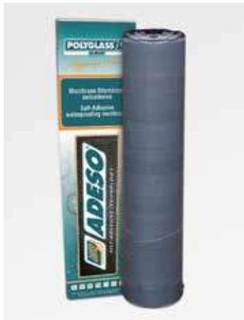
POLYVAP SA is a prefabricated double-sided self-adhesive bitumen membrane produced using ADESO technology, made up of a special self-adhesive elastomeric compound (SBS) reinforced with an aluminium foil. For use as a vapour barrier, it meets the requirements of standard EN 13970. Its use is recommended in all cases where application not involves torching.
