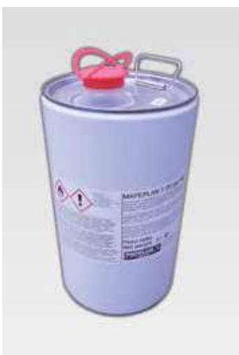
MAPEPLAN T SEAM PREP is an organic-solvent-based liquid cleaner specially formulated for preparing overlaps prior to welding of MAPEPLAN T FPO/TPO waterproofing membranes, to be used to boost the membrane weldability properties.
