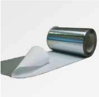
BUTYLSTRIP is a high-adhesive butyl sealing tape protected by a reinforced aluminum film. The aluminum film gives to the product resistance to ageing, to oxidizing and to the aggression of chemical and atmospheric agents. It is cold applied, waterproof and self-sealing, features good adhesion at low temperatures and heat stability, does not release oily substances and is solvent free. It can be used for daily provisional waterproofing sealing jobs.
