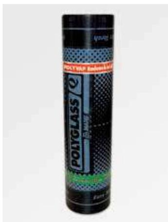
POLYVAP RADONSHIELD is a prefabricated waterproofing elastomeric-plastomeric membrane, with a distilled bitumen-based compound modified with polypropylene, reinforced with a 6/100 thickness aluminum strip bonded to reinforced glass fibre.
