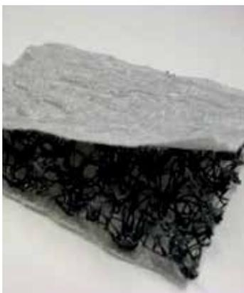
POLYSTUOIA 20 and POLYSTUOIA 20L are protective and drainage geocomposites comprising two UV-stabilized, needle-punched polypropylene staple-fibre filter geotextiles with a 3-dimensional drainage structure sandwiched between them made up of polypropylene monofilaments. The two geotextiles are heat bonded to the drainage core using a continuous process.
