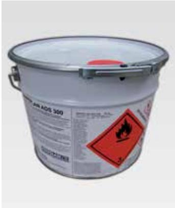
MAPEPLAN ADS 300 is a polichloroprenic monocomponent solvent adhesive for double coating (contact adhesive), designed to bond MAPEPLAN T B membrane on vertical surfaces.
