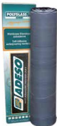
POLYVAP SA is a prefabricated double-sided self-adhesive bitumen membrane produced using ADESO technology, made up of a special self-adhesive elastomeric compound (SBS) reinforced with an aluminium foil. For use as a vapour barrier, it meets the requirements of standard EN 13970. Its use is recommended in all cases where application does not involve torching.
