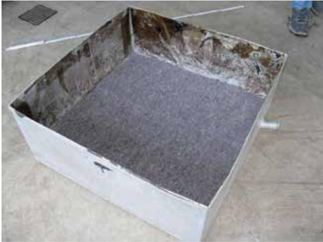
The FLL test consists in lining eight boxes measuring 80x80x30 cm with the root-resistant membrane to be tested.
