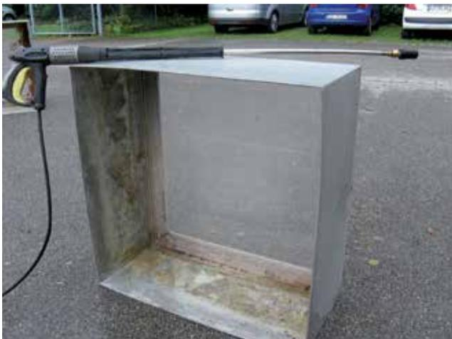
The bottom of the box is transparent, being made from Plexiglas, to allow for visual inspection at six-month intervals (to see whether roots have gone through the membrane).
