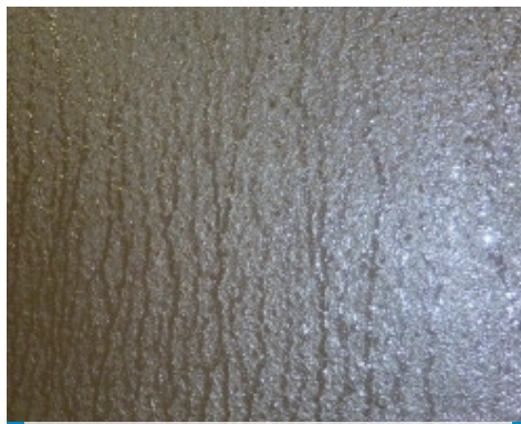
Normal bleeding on the surface of the product immediately after application
